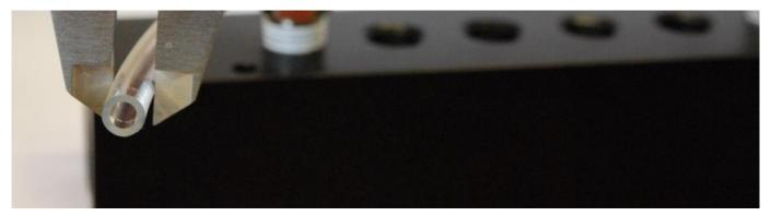
The Outer Diameter measurement on Push To Connect Fittings is used to identify which kind of tubing it matches. For example the MTU 1/4 features 1/4" Push To Connect sleeves that are suitable for 1/4" OD tubing. All MettleAir fittings feature raised number that allow users to easily identify the OD sizing on the easily recognizable blue push to connect sleeve.
