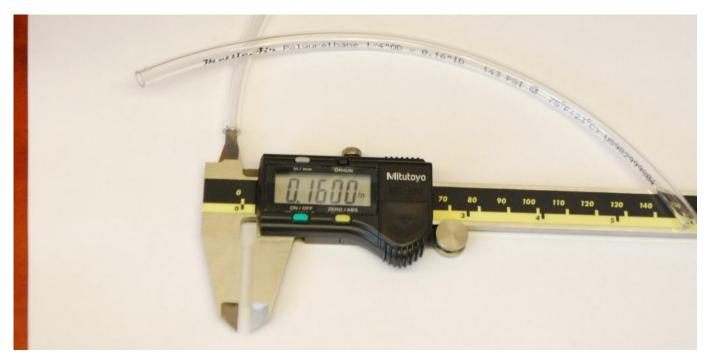
The Hose ID/Interior Diameter measurement on brass barbed fittings is used to identify which kind of tubing it matches. For example the 125-2B features a 1/8" Hose ID end that is suitable for 1/8" ID (0.16" ID) tubing. Below is how you measure Hose ID off your existing fitting, notice how we used the very tip of the brass fitting and that it is acutally measuring the inner most points of the barb's exterior/tip. (Degree of tolerence varies between tubing and fitting).
